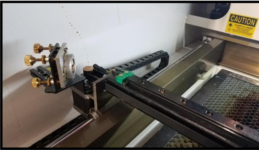
The beam emits from the tube onto a mirror positioned at a 45-degree angle. The 2<sup>nd</sup> mirror (mounted to the gantry shown at left) catches the beam and projects it across the machine to the 3<sup>rd</sup> mirror mounted in the laser head.
